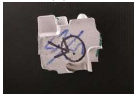
Fig 6: Blow-hole defect cut piece.
