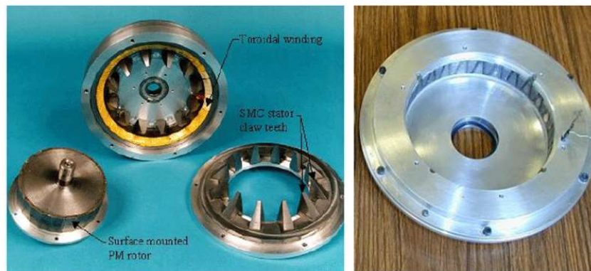
(a) Jack's single sided 'claw pole' MPM [29] machine [36]
