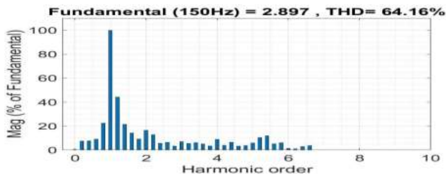
Fig. 18: Frequency Spectrum of Current at 1.5Nm Load.
