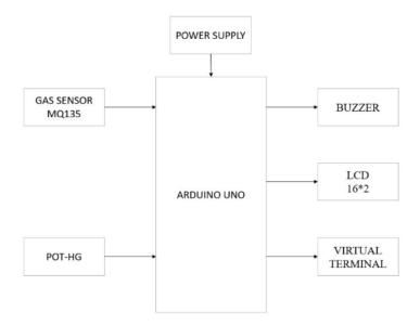
The data of air is recognized by the MQ135 gas sensor. The MQ135 sensor can sense NH3, NOx, alcohol, Benzene, smoke, CO2. So, it is a dynamic gas sensor for our Air pollution Monitoring system. When it is connected to Arduino then it will sense all gases, and it will give the Pollution level in terms of PPM (parts per million).
