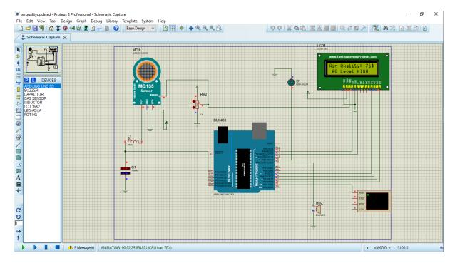
If the ppm is less than the threshold value, Then we turn off LED, and Buzzer turns on and prints "AQ LEVEL LOW" If its high particulate matter is high and the air is impure and no need to be purified.
