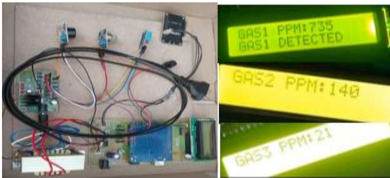
Fig 2. Hardware setup and MQ sensors outputs
