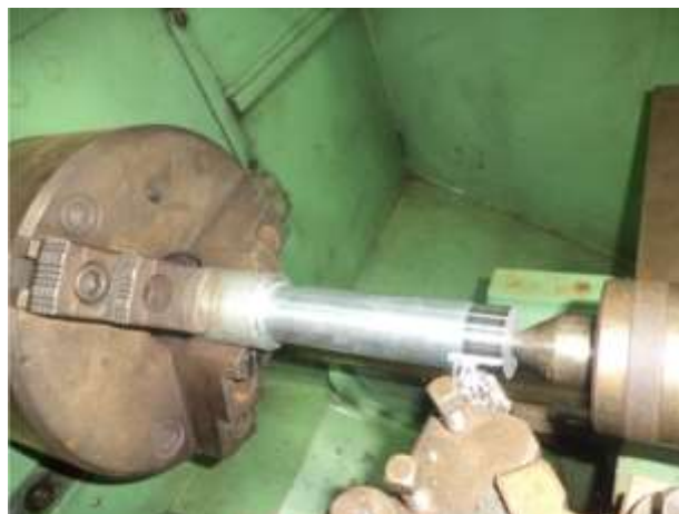
Fig. 1 Experimental setup during turning the Al 7075 alloy
