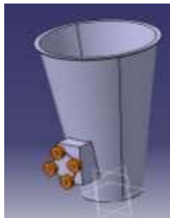
Fig. 4.3 3D cad model of bucket with rollers
