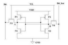
Fig4: Schematic of 6T SRAM Cell
