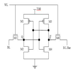
Fig2: 6T SRAM Cell (Traditional)
