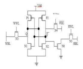
Fig 3:8T SRAM Cell
