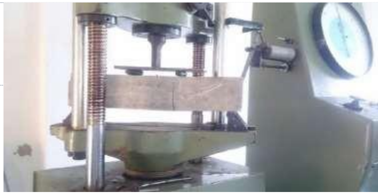
Figure. 2: Specimen loading for flexural strength test
