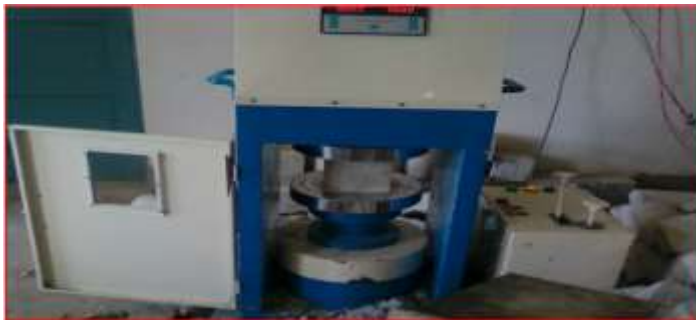
Figure 2: Cube specimen loaded in compression testing machine
