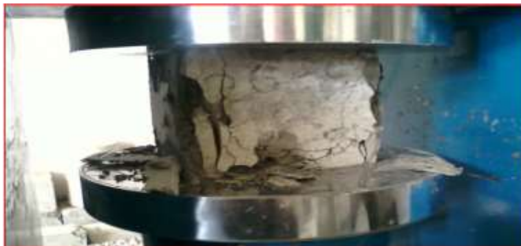
Figure 3: Cube specimen after failure
